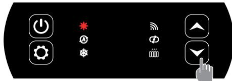
With the heat pump on, press on for 5 seconds to start the WiFi pairing. The WiFi logo flashes.
