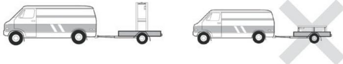
The equipment must always be stored and transported vertically on a pallet and in its original packaging. If it is stored or transported horizontally, wait at least 24 hours before switching it on.
